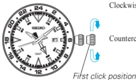
Clockwise: the hour hand turns counterclockwise. The date is set back one day when the hour hand makes two full rotations counterclockwise.
