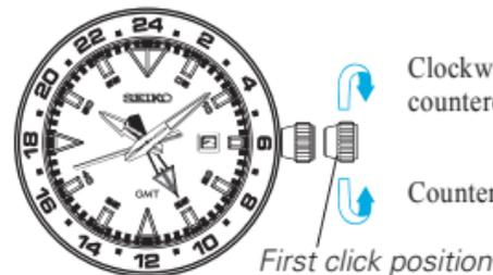
Clockwise: Setting the time back (The hour hand turns counterclockwise.)
