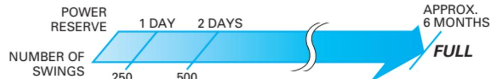
1. When the watch stops completely, or if you find the second hand moving at two-second intervals, swing the watch from side to side at a rate of twice a second.
