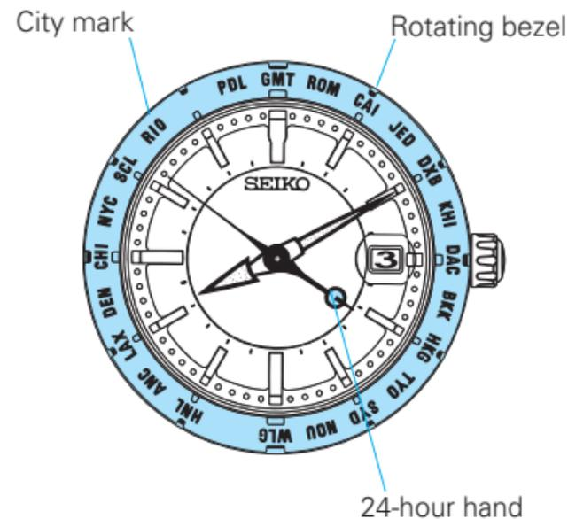
Turn the rotating bezel so that the city mark corresponding to the area whose time has been set in the "How to set the time" aligns with the 24-hour hand.
