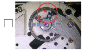
2) Push out the stud parallel to the slit of the STUD SUPPORT (the direction also shown by the red arrow in the illustration) in order to remove it from the STUD SUPPORT.
