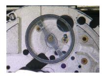
2) Set the BALANCE COCK WITH REGURATOR and tighten the BALANCE COCK SCREW.
