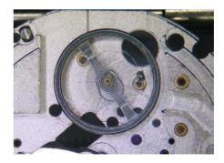
4) Remove the BALANCE COMPLETE WITH STUD.
