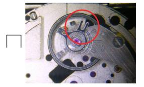
3) Unscrew the BALANCE COCK SCREW and remove the BALANCE COCK WITH REGULATOR.
