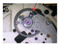
5) Engage the balance-spring with the slit of the REGULATOR PIN.
