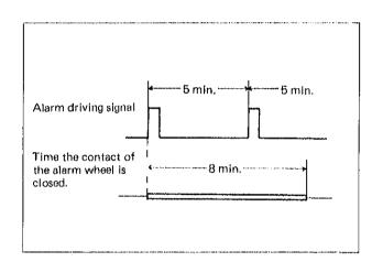
To remove the possibility of this delay, it is therefore required to put the hour and minute hands at the position 3 minutes short of the 12 o'clock position so that the alarm may ring correctly at any position where the alarm time is set, even if the time to close the contacts of the alarm wheels shifts more or less.
