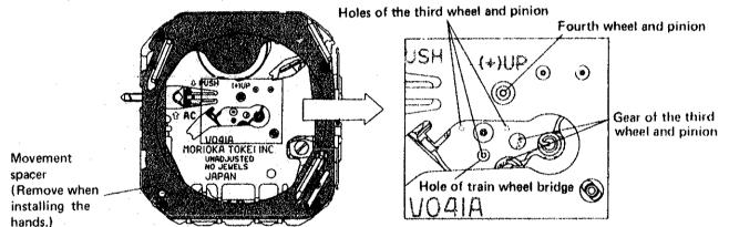
3. Be sure to install the hour, minute and second hands so that they point exactly to the 12 o'clock position.
