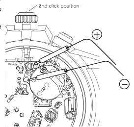
\* When measuring the voltage using the SEIKO digital multi-tester (S-860), use the range of V.
