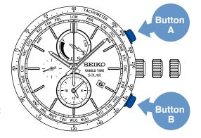
Resetting the IC will initialize the watch. Before starting to use the watch, it will be necessary to set the time and date after adjusting the preliminary position of the Chronograph hands (second, hour and minute) and mode indicator. Refer to the following sections in the instruction booklet.
