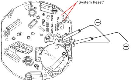
\* When measuring the current consumption using the SEIKO digital multi-tester (S-860), use the range of 40 μA of SUPPLY V (=1.55 V) & GATE TIME (2S).
