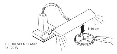
**Note:** In case the measurement of the voltage for the watch does not achieve the standard value but the measurement for the solar cell unit alone exceeds the standard value, a problem in the electrical conductivity between the solar cell unit and the movement is suspected. Inspect the electrical conductivity, especially at the CONTACT SPRING FOR SOLAR CELL, and check the solar power generation system again.
