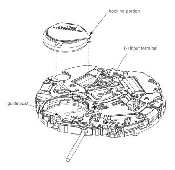
\* Slide the Rechargeable Battery Block under the hooking portion of the Rechargeable Battery Guard if it is after setting the Rechargeable Battery Guard.
