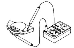
$120\Omega \sim 140\Omega$ : Normal Less than 1200: Short circuit (Defective)
