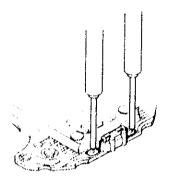
Lights up: Normal Proceed to Does not light up: Defective Replace the bulb with a new one.
